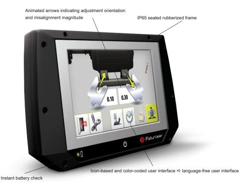
Integrated Bluetooth for wireless communication between display unit and smart sensors
